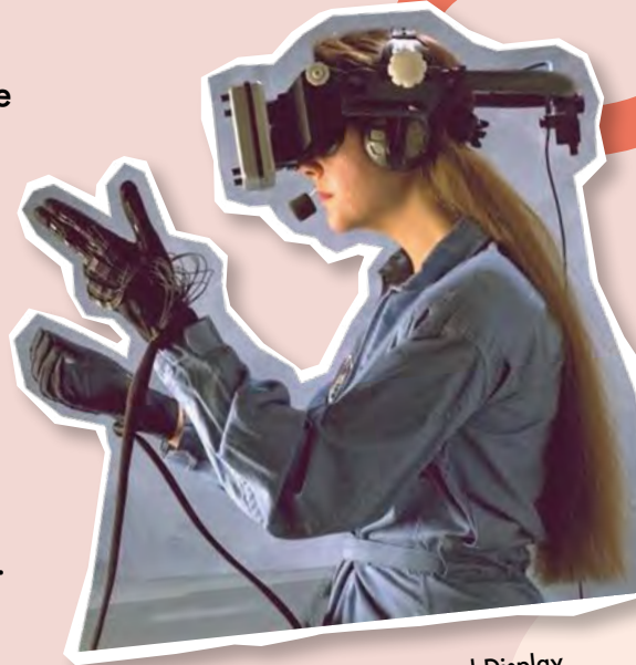
Zestaw HMD – Head Mounted Display i cyber rękawice z Ames Research Center NASA
